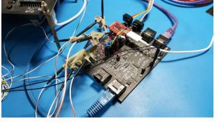
Here is the very small (4x3 module) subset of a display under construction and the first live video from a Windows notebook. Moire is an artifact of image capture, view at large size for better appearance.
