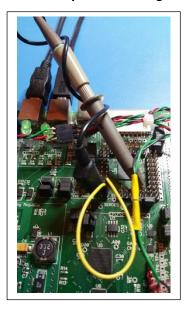
Node 705 of the target chip was programmed to produce a relatively low frequency (10 Mwords/sec) stimulus consisting of two data bits and a clock, using the code shown above, and jumpers used to carry its signals to nodes 008 and 007 as shown to the left.
