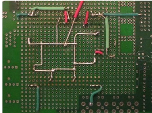
Finally, Mark arranged for five signal and ground pairs connecting to GA144 pins 708.17 and 708.1 for asynch boot and to 300.17 and 300.1 for synchronous boot, with one more pair to pin 88 for RESET-. These pairs were secured and terminated with Berg pins crimped to the ends of the stranded wires and surrounded by short pieces of heat shrinkable tubing. The resulting modified Evaluation Board is shown below.
